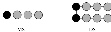
Figure 1. Schematic models of MS and DS. Counterions are not shown. ● :head group; ○ :tail group.
